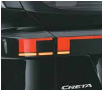
LED rear turn signal with sequential function
