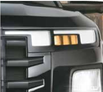
Front turn signal with sequential function
