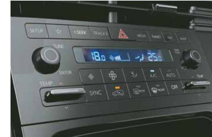
Dual zone automatic temperature control (DATC)
