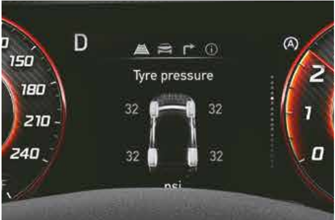
Tyre pressure monitoring system: Highline
