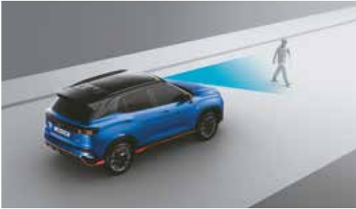
Forward Collision - Avoidance Assist - Pedestrian (FCA-Ped)
