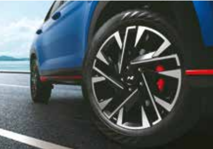
R18 (D=462 mm) diamond cut alloys with N logo and red caliper
